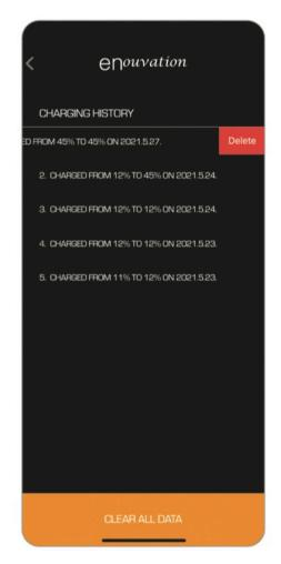
To delete an entry, swipe to the left to reveal a delete button. Tap delete to remove it from the list.
